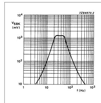
Fig.2 BK signal voltage at pin 5 as a function of frequency.
