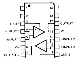
Pin 6 connected to bottom of package.
