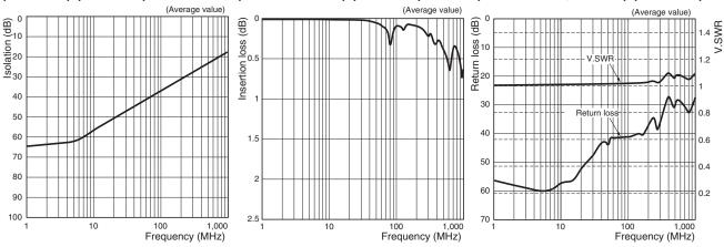
Note: High-frequency characteristics depend on the PCB to which the Relay is mounted. Always check these characteristics, including endurance, in the actual machine before use.
